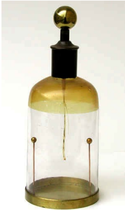
first gold leaf electroscope built by Abraham Bennet in the 1700s
