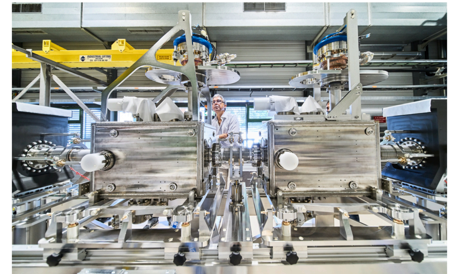
Assembly of two crab cavities for the High-Luminosity LHC (Image: Julien Ordan/CERN)
