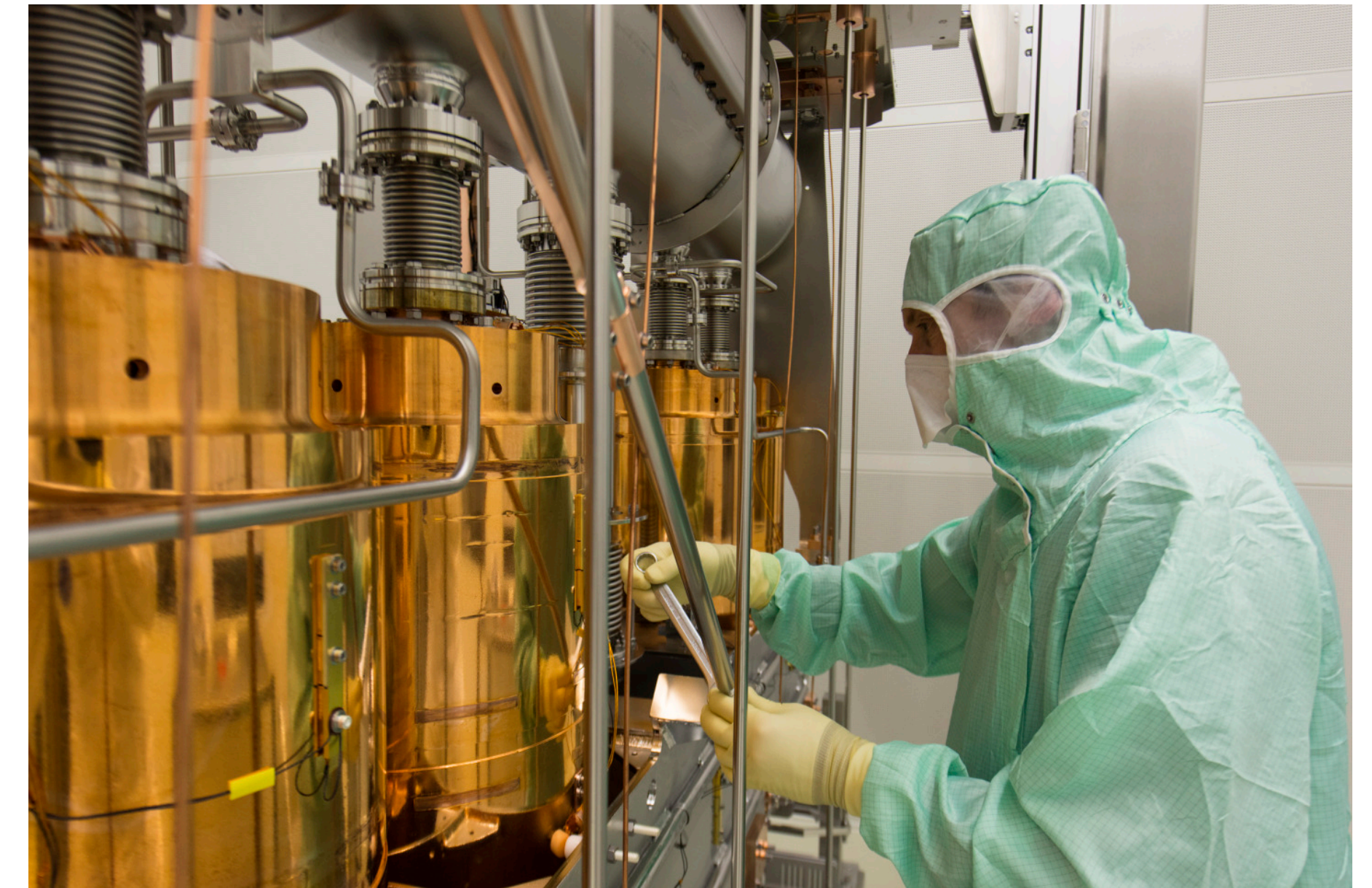
Assembly of cavities for the HIE-ISOLDE accelerator (Image: Maximilien Brice/CERN)
