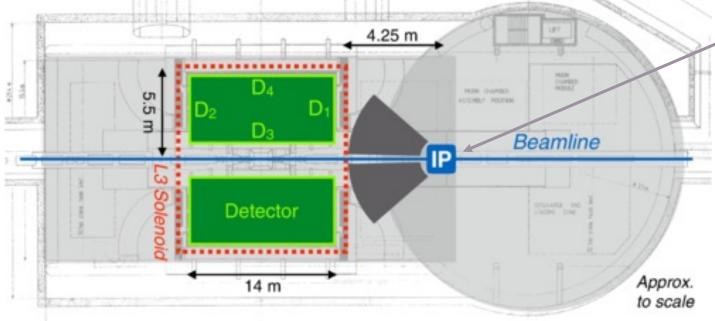
ALICE interaction point moved by 11.25 m outside magnet to allow LLPs to travel before decaying
