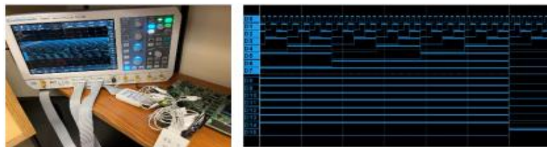
Outputs from eFPGA (16b counter) probed with oscilloscope
