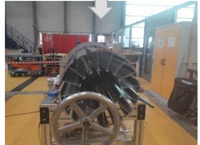
Insertion of each PM blocks (16 segments per row). 12 rows for the 1-m long version and 18 rows for the 1.5-m long version.
