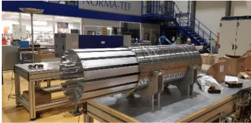
Assembly of the dipole yoke including steel ring and aluminium profiles.
