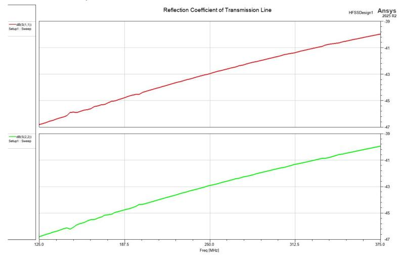
•  $S_{11}$ ,  $S_{22}$  = -40dB => 0.01 that means 1% of input signal reflected on Port 1 and Port 2 respectively.
