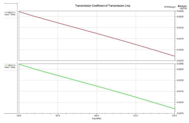
•  $S_{21}$ ,  $S_{12}$  = -0.03250dB => 0.9962 that means 99.62% of input signal is transmitted from Port 2 to Port 1 and vice versa.
