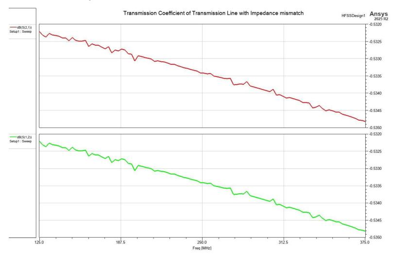
•  $S_{21}$ ,  $S_{12}$  = -0.5340dB => 0.9404 that means 94.04% of input signal is transmitted from Port 2 to Port 1 and vice versa.
