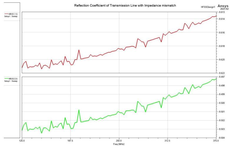
•  $S_{21}$ ,  $S_{12}$  = -0.03250dB => 0.3306 that means 33.06% of input signal reflected on Port 1 and Port 2 respectively.
