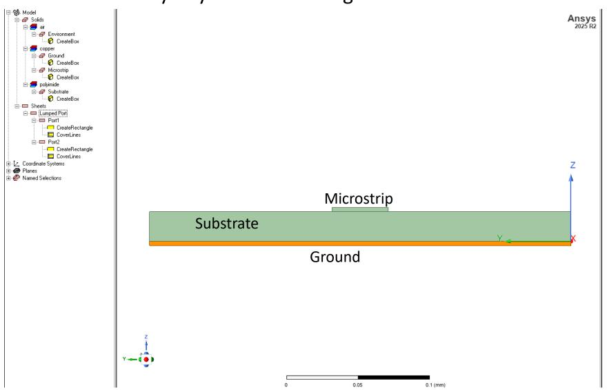
• Step 2: Create Port plane perpendicular to Microstrip on both ends.
