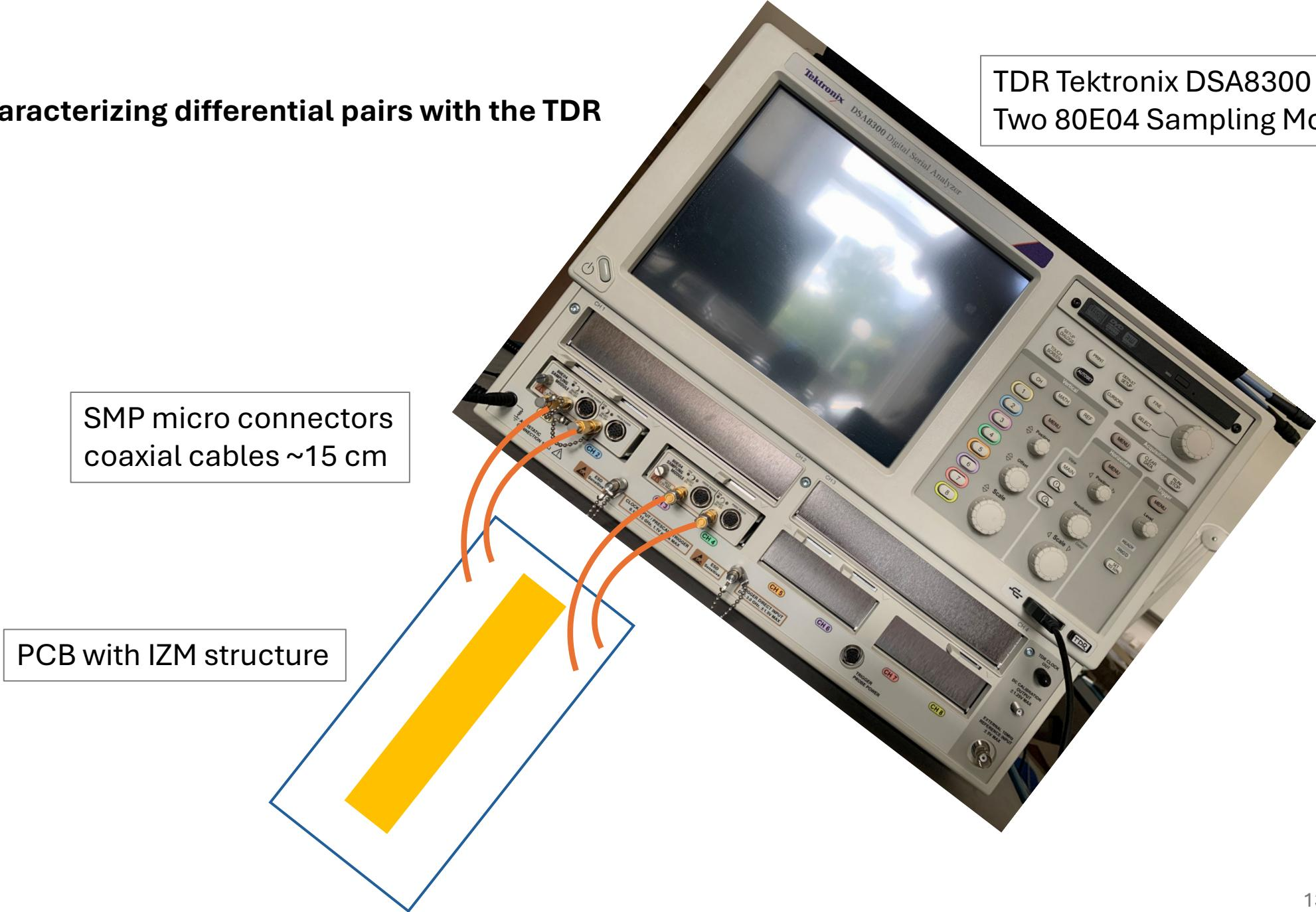
We will use a microwave small size connector of SMP type to allow for shorter traces on the PCB
