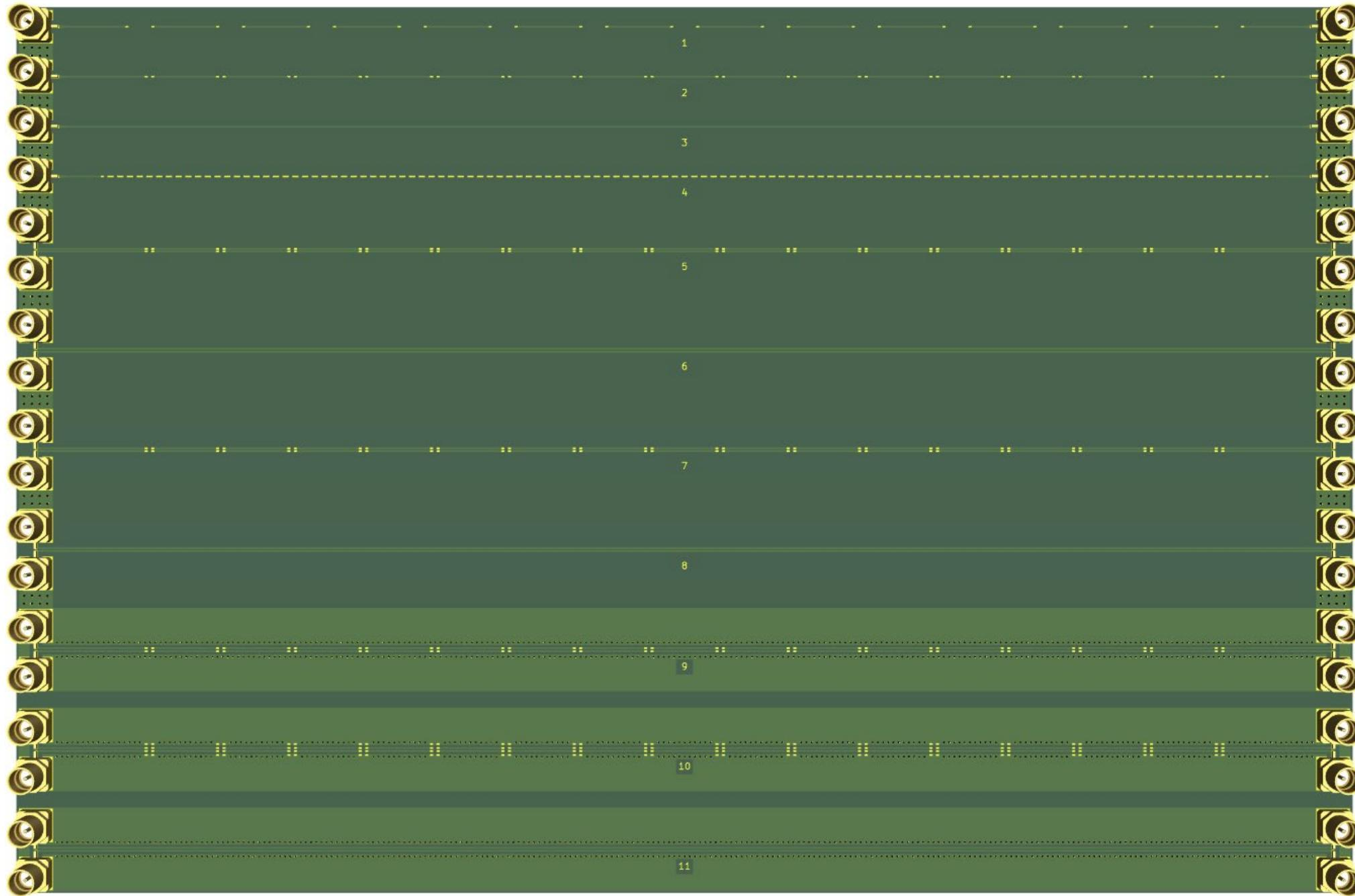
This is our preliminary PCB design for hosting the structure and interfacing with measuring devices:
