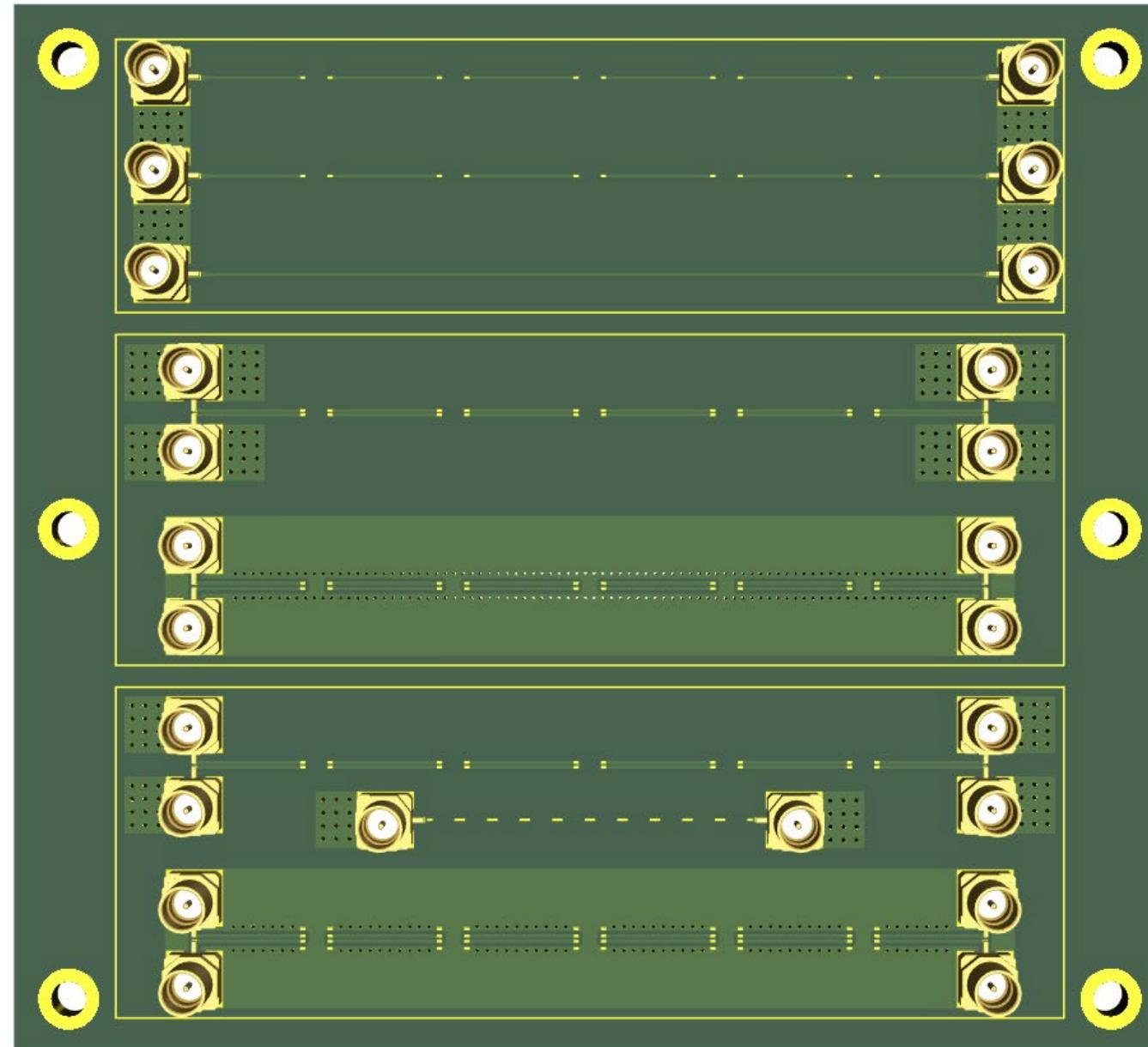
We will use a microwave small size connector of SMP type to allow for shorter traces on the PCB
