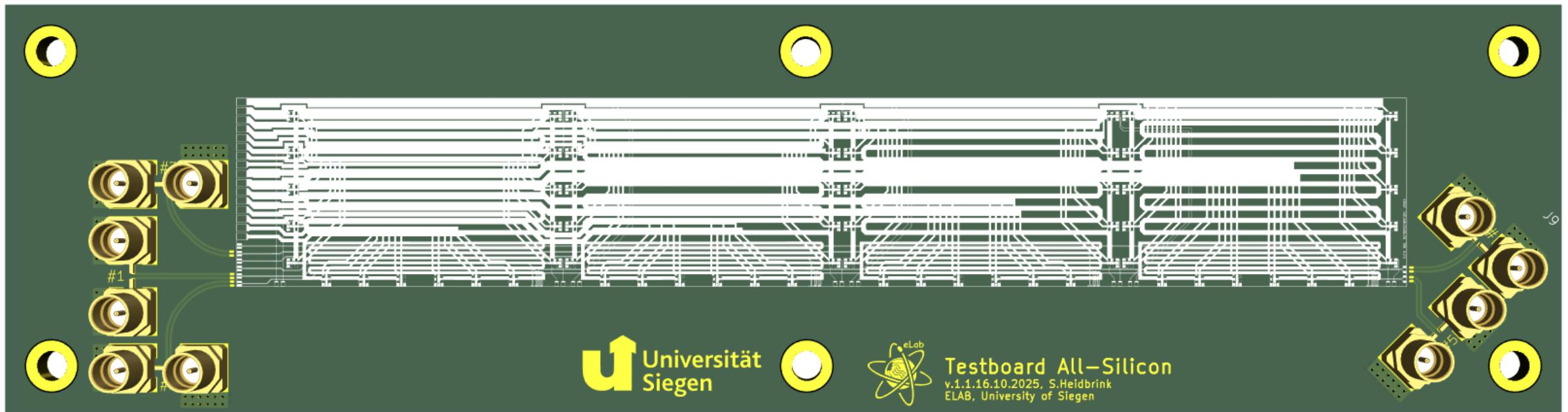
This is our preliminary PCB design for hosting the structure and interfacing with measuring devices:
