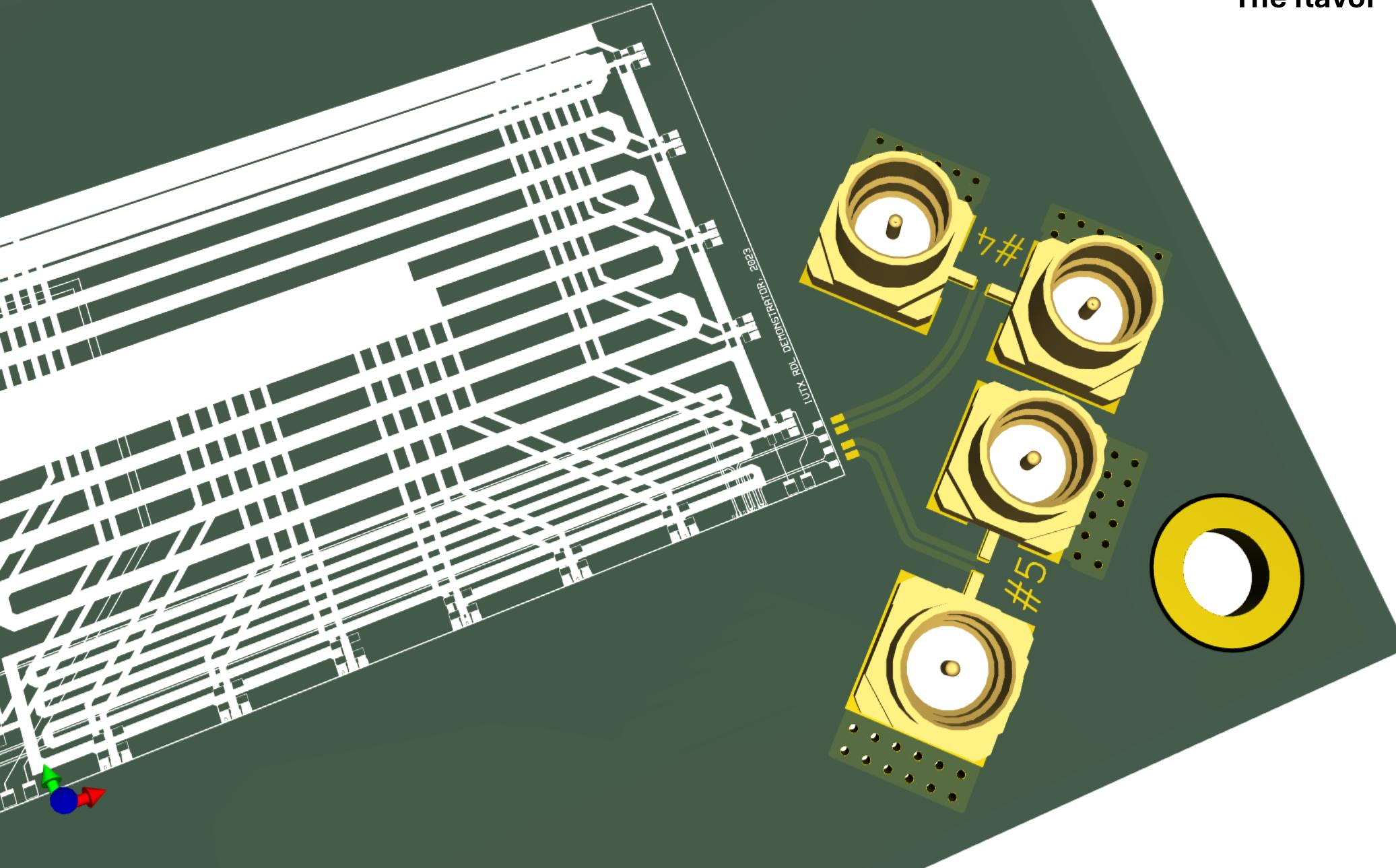
This is our preliminary PCB design for testing and studying the impedance matching of the wire bonds
