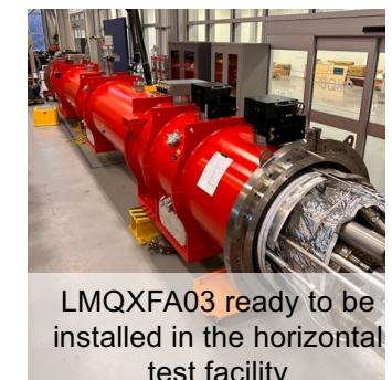
LMQXFA03 ready to be installed in the horizontal test facility
