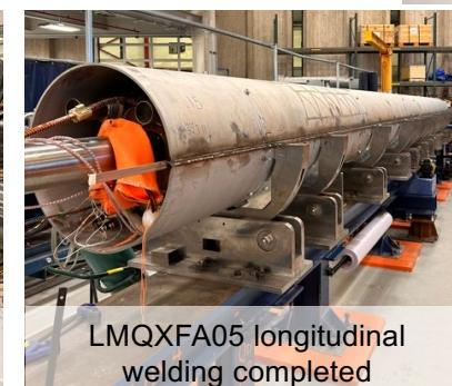
LMQXFA05 longitudinal welding completed
