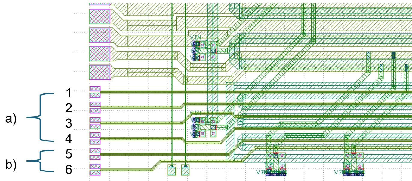
**E1 to E6 labels** mark endings of the six differential transmission line pairs
